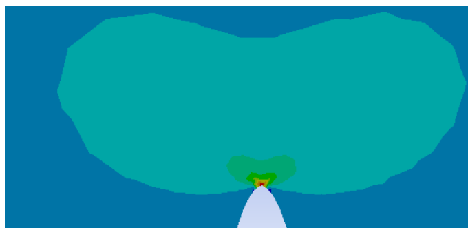
Fig. 6. – Normal (horizontal) stress distribution at the top of crack
